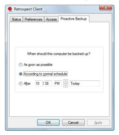
These controls let the user affect when the client computer can be backed up by the backup computer (using a Proactive Backup script). The user would normally use it to request a backup or defer a backup, but the user can also revert Proactive Backup back to its normal schedule for this client. The Proactive Backup options are:
